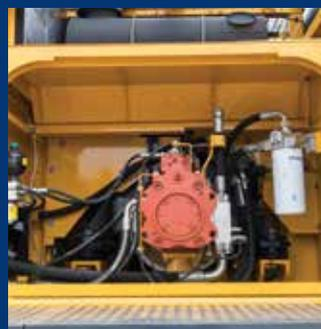
The 995F's advanced variable hydraulic control system allows the machine to change the pressure and distribution of flow according to the application and conditions helping to improve efficiency, productivity, and durability.
